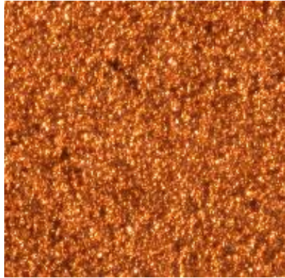
Base Cu electroplated surface
